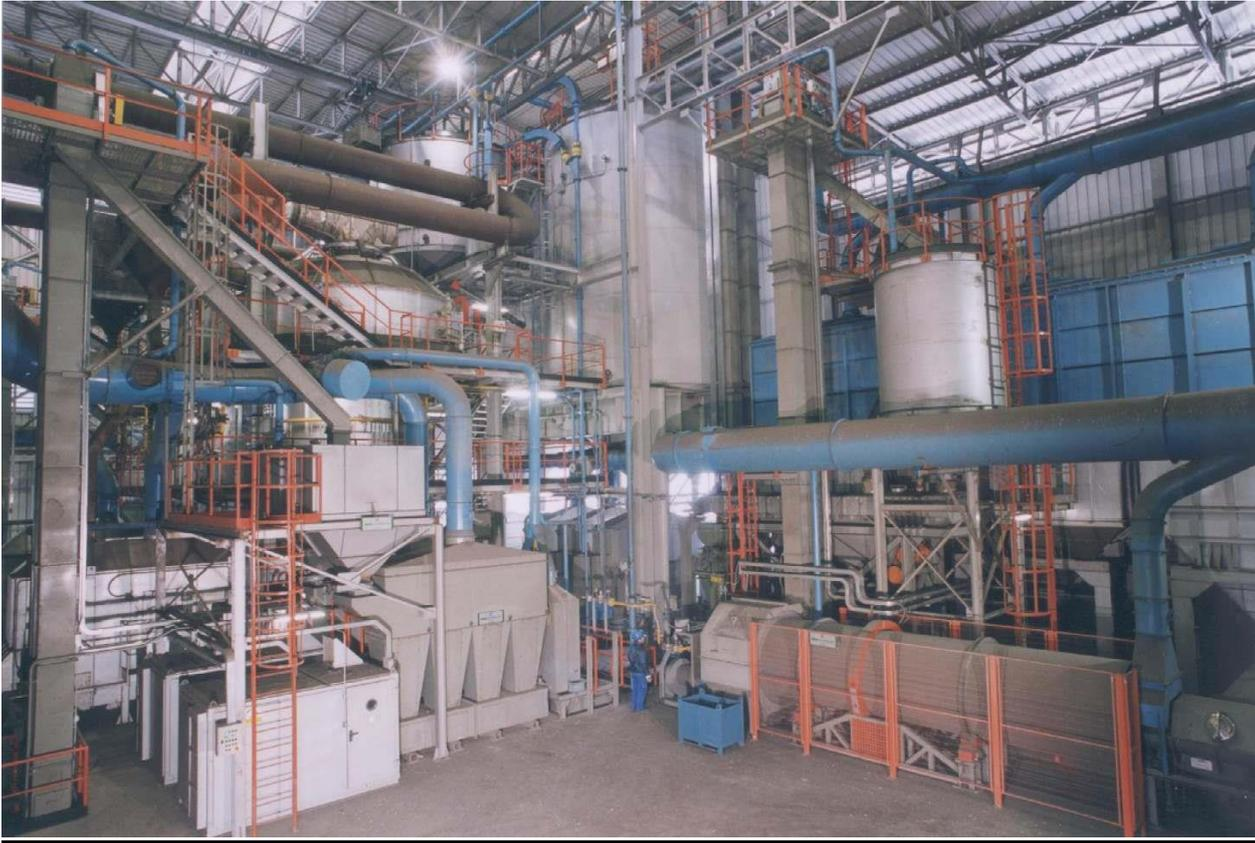
**Project Requirement:** The customer had a green sand regeneration requirement of approximately 14 ton/h coming from a mold line used mainly for producing cast iron motor blocks.
